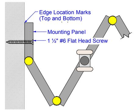
Insert 1 1/2" #6 flat head screws about 8" up from the floor and 8" down from the track.
