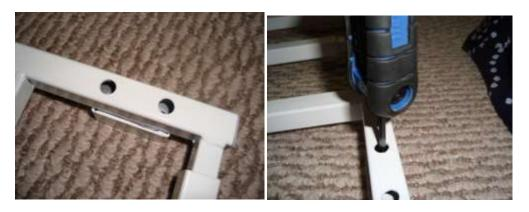
Step 5 Lock is in place now. Check Lock by inserting lock bracket (On Angle frame), Locking and un Locking
